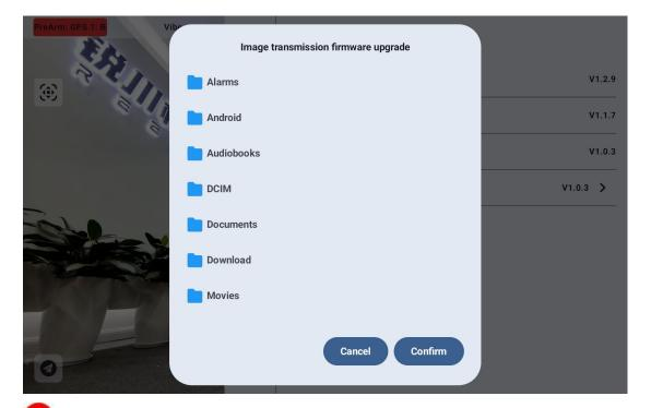
**Note:** The firmware of the graphic transmission module at the air unit and the ground end needs to be the same version before communication can be carried out.
