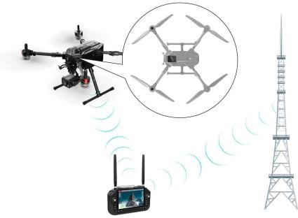
Use the handheld ground station to run the Mission Planner ground station software and connect the handheld ground station to the mobile Internet. Go to Initial Settings> RTK > NTRIP ".
