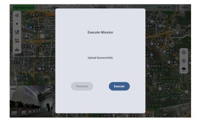
• Manually unlock the aircraft, the drone will automatically perform route tasks
