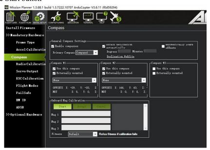
• Lift the drone and rotate it in different directions so that each side (front, back, left, right, top and bottom) points down to the earth for a few seconds
