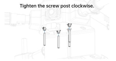
Mount the optical pod onto the expansion board.
