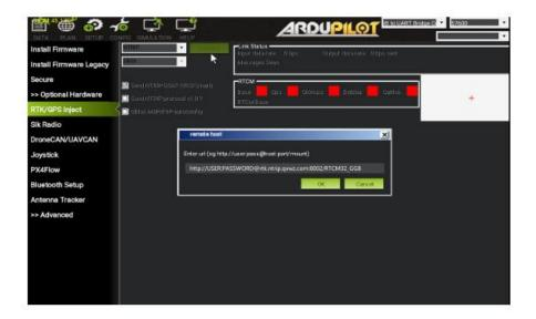
Among them, USER is the FindCM service account name applied by the user, PASSWORD is the corresponding password, rtk.ntrip.qxwz.com is the FindCM service address of qianhe location server, 8002 port broadcasts WGS84 coordinate system data, and RTCM32\_GGB is the data source for externally broadcasting RTCM3.2 format data.
