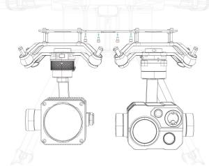
Thread the cable through the rubber plug into the fuselage.
