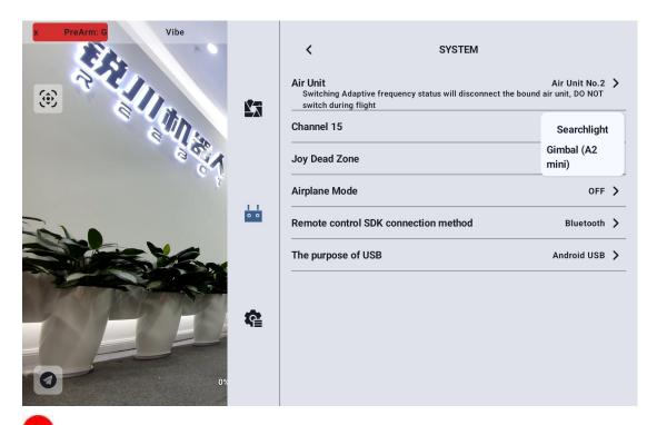
Note: Channel 15 corresponds to the equipment connected to LAN 1 interface at the air unit, channel 16 corresponds to the equipment connected to LAN 2 interface at the air unit, and channel 16 defaults to searchlight
