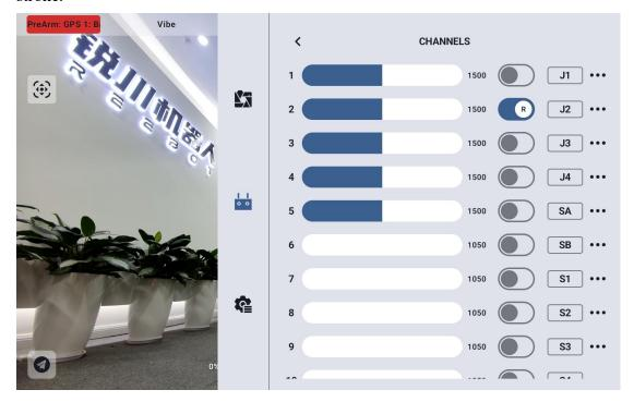
Select the target channel and click the corresponding steering gear forward and reverse switch to successfully set the steering gear forward and reverse.
