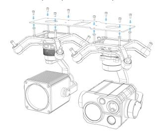
Secure the expansion board to the screw post.
