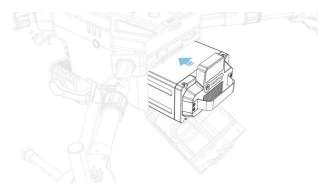
Check the power: short press the battery power button once
