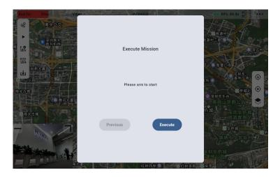
• At the end of the mission waypoints, add the appropriate waypoints to guide the aircraft back to the landing point on a safe path.
