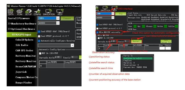
It is recommended to check the automatic configuration F9P, set the observation accuracy to 2.5, and set the minimum observation time to 60s.
