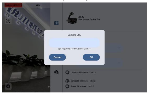
Note: When two gimbal platforms are connected at the same time, the IP address of one of the gimbal platforms needs to be changed to the end of non -25. When connecting, choose to manually enter the rtsp address to connect
